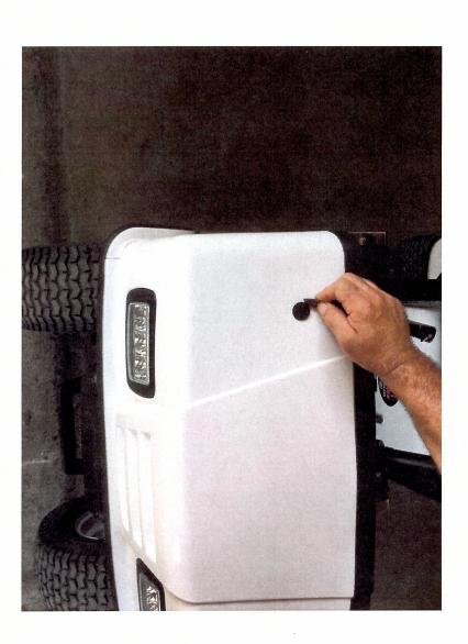
Remove black caps in front cowl Insert aluminum spacers into hole where caps were Lay plastic bushing over hole in cowl with long end to rear of Cricket
