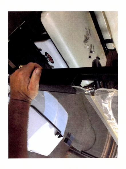
windshield clips onto front frame until they snap on frame Now tighten all nuts & bolts Make sure all parts look square and straight, Line up windshield long clips after installed , to front u shaped windshield frame , push long
