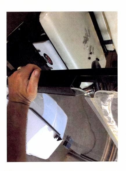
windshield clips onto front frame until they snap on frame Now tighten all nuts & bolts Line up windshield long clips after installed , to front u shaped windshield frame , push long Make sure all parts look square and straight,
