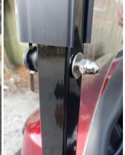
7. Install top frame with rear view mirror mount towards front of cart to the front vertical rail by aligning front holes in top frame with the and loosley attaching hardware show below. Do the same to the other side.
