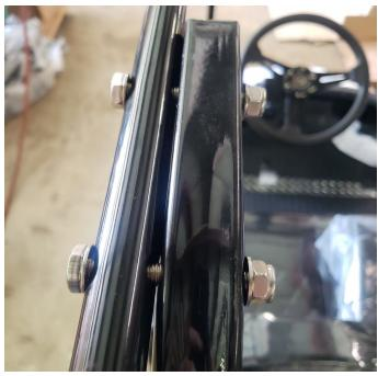
9. Tighten all hardware & knobs that were left loose, then install screw for cover on front vertical rail as shown below.
