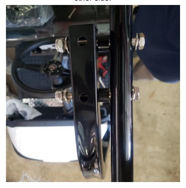
8. Install top frame to the rear vertical rail by aligning rear holes in top frame with holes in rear vertical rails and loosely attaching hardware show below. Do the same to the other side.
