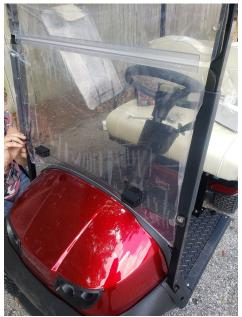
6. Slide windshield up or down until the hole in the rubber grommet matches hole in front vertical rail.
