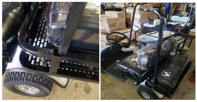
4. Install front rail cover by sliding down from the top of rail as show in picture below to both sides.
