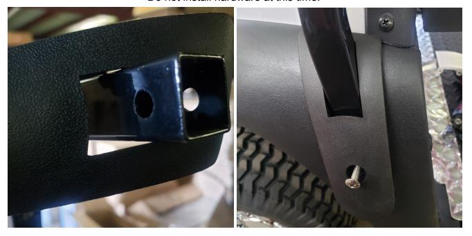
5. Install the black plastic clips and rubber grommet to each side of windshield. Then align black plastic clip with each front vertical rail and snap in place.
